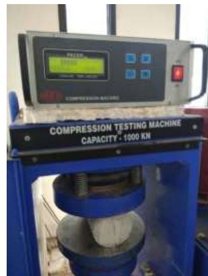
Fig.2. Split Tensile Strength test of cylinder
