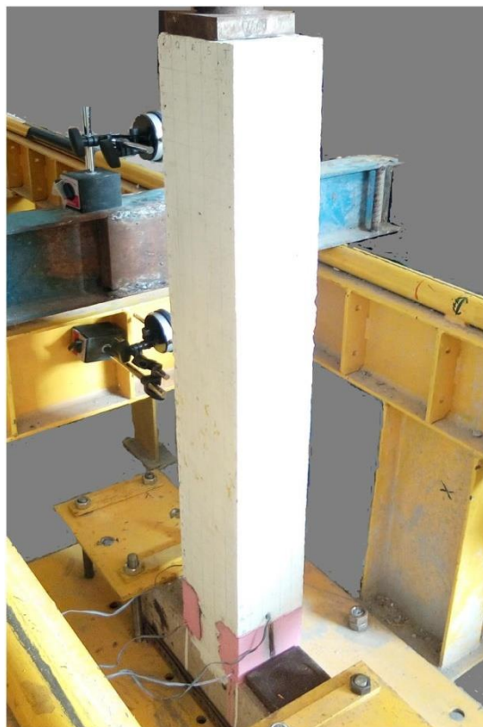
Fig. 2 Fitting the RC column specimen to restrain translation and rotational movement at the beam-column joint
